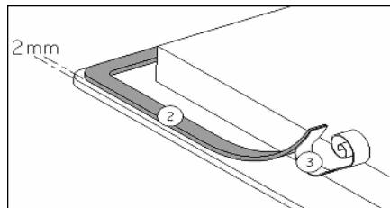
Glue the seal (2) two millimetres from the outer edge of the glass after removing the protective film.
